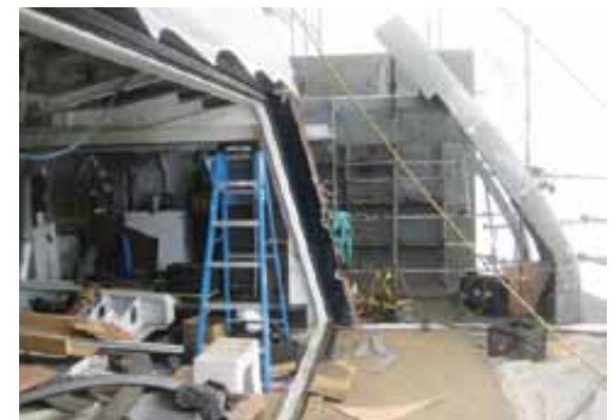
ABOVE: PROVIDING BETTER ACCESS TO THE WATER AND TENDERS WAS AN IMPORTANT PART OF THE REFIT AND ADDED THREE METRES TO THE YACHT’S LENGTH. THE SIDES OF THE AFT HULL WERE EXTENDED AND WRAPPED AROUND THE BATHING PLATFORM AND GARAGE OPENING TO GIVE GUESTS AN EASIER ROUTE TO THE STERN FROM THE AFT DECK
